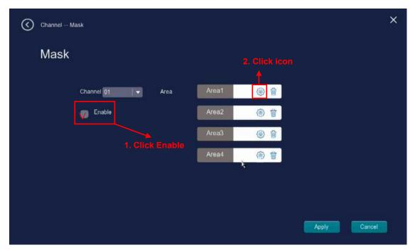
This page is used to Adjust the occlusion area of the monitoring channel.
